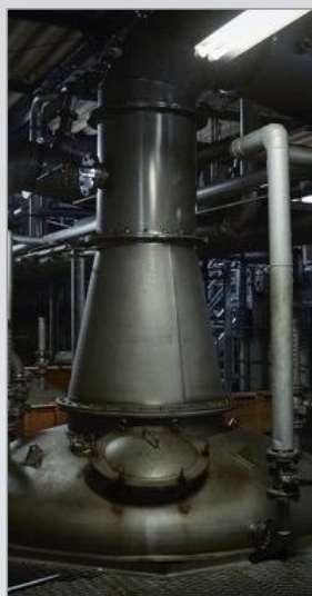
Koji mash distilled in pot stills at Osumi Distillery
