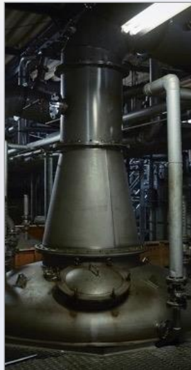
Osumi Distillery: Koji mash distilled in pot stills
